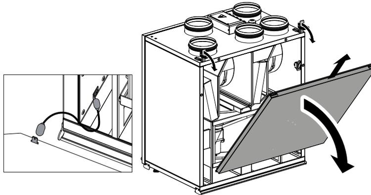
3. Remove the latches and move them to the opposite side. Remove the back panel by undoing the four screws.
