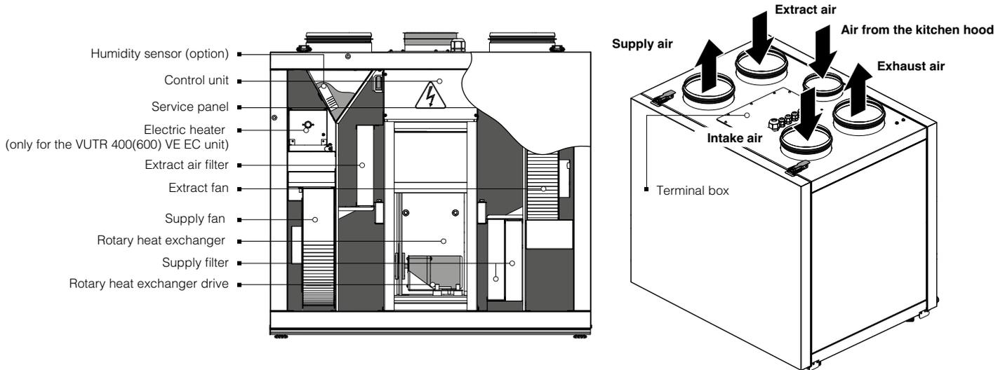
An exhaust kitchen hood may be optionally connected to the unit. The kitchen hood must be equipped with an air damper to shut off the exhaust duct when the kitchen hood is not in use.
