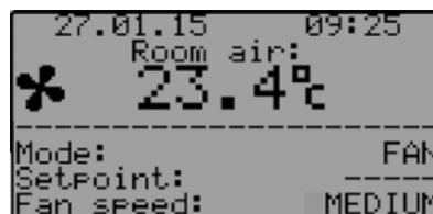
Fan speed control in the **Auto mode** requires a th-Tune control panel in a special configuration or with an external humidity sensor with a 0-10 V output signal. Enable the «**Humidity feedback speed control**» and set the maximum and minimum speed for the supply and exhaust fans as a percentage value. Set the «**Auto**» fan speed.
