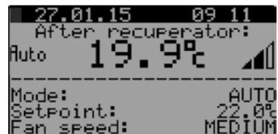
**5. Temperature at defrosting sensor.** The feedback is provided by the temperature sensor installed on the heat-transfer unit of the exhaust air duct.
