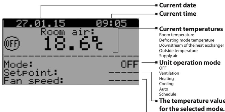
When using the th-Tune control panel the screen has a different configuration, but all the readings and settings are identical.
