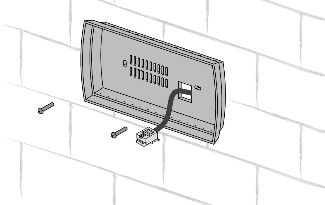
2. Connect the phone cable to the front part of the control panel. Install the front part of the control panel into the box by fastening it to the rear part of the casing with countersunk screws supplied as shown in the figure below and then install the front bezel by pushing it until it clicks in position.
