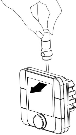
2. Disconnect the 4-pin socket from the front part of the control panel.
