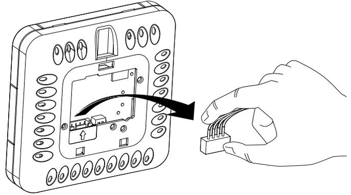
3. Complete the electrical connections according to the external connection diagram (Page. 14 ).
