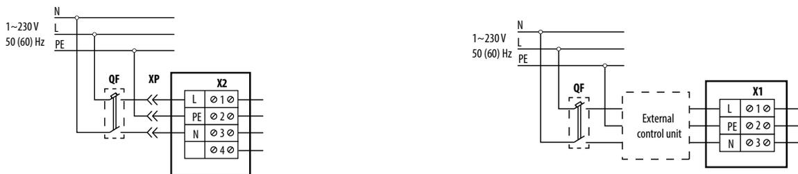
The fan is connected to power mains by means of the power cable only in a remote terminal box (X1)
