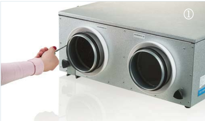
Cover the air handling unit spigots with the flanges from NM Isovent mounting kit and fix those with self-drilling screws with drill.
