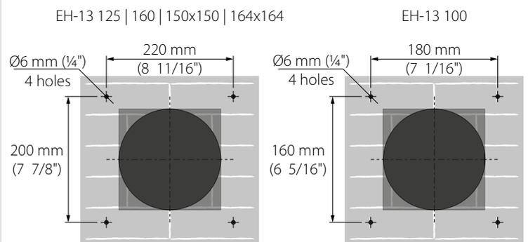
3. Insert the supplied expansion anchors 6 mm (1/4")x40 mm (1 9/16") into the holes.
