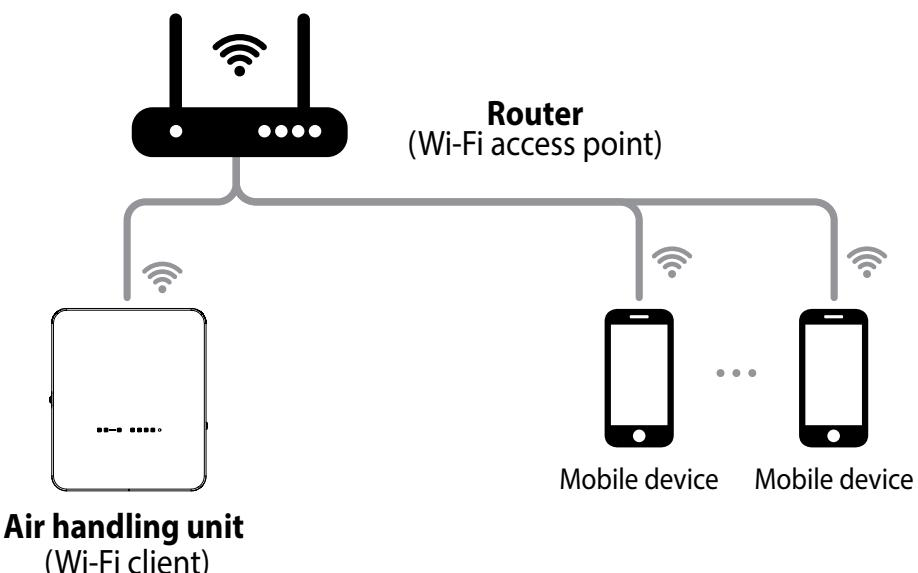
**Example 3:** Smart Home system connection via router with several Wi-Fi access points.
