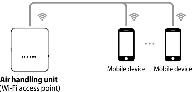
**Example 2:** connection via router with one Wi-Fi access point.
