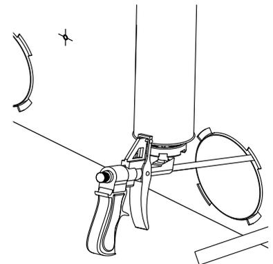
**5.** To install an additional extract spigot, remove the plug on the rear part of the unit. Undo the screws, remove the plug and fix a spigot on its place using screws.
