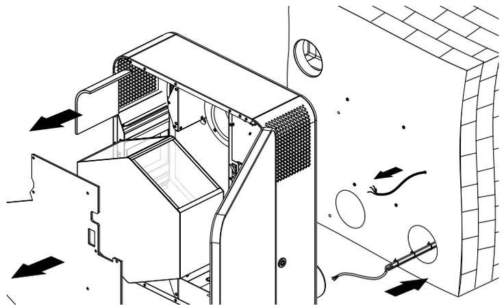
**7.** Install the outer ventilation hood:
