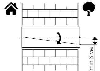
**4.** Fill the spaces between the air ducts and the wall with a mounting foam through the specially designed holes in the mounting template.
