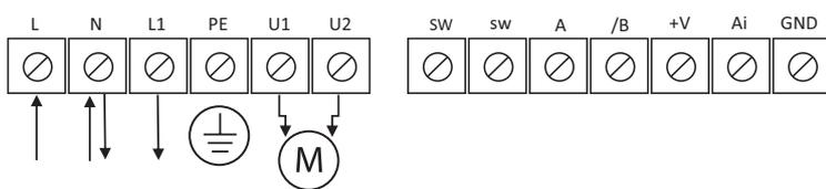
**Wiring diagram and connections**
