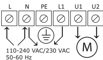
Controller wiring diagram
