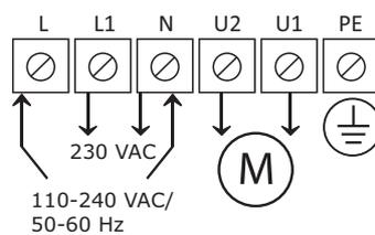
Controller wiring diagram
