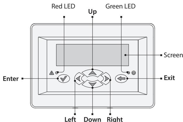
Fig. 2 Control panel button functions
