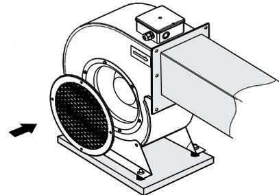
**After installing the unit, you need to make sure that the fan impeller rotates freely.**
