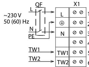
**3. VCU(z) with a magnetic starter and a thermal switch**
