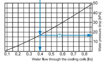
**How to use water cooling coils diagrams**
