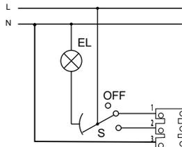
External switch **S** (e.g. P2-1-300) is used to set the fan to one of the two available speeds simultaneously with switching on the lights in the room or disable the fan when the lights are switched off. The fan is enabled/disabled simultaneously with the lights only.
