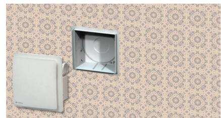
The fan casing is mounted during construction works. Electric wiring for connection of the VNV-1A(E) 80 ventilation unit is led out through a special hole in the casing. The front panel is covered with the protective cardboard plate supplied with the unit to avoid damages or contamination during finishing works in the room. After finishing the works the protective cardboard plate is removed and the VNV-1A(E) 80 ventilation unit is installed into the casing that is connected to the wiring.
