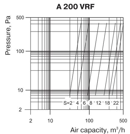
The internal part of the air disk valve is pulled out to ensure the required clearance S mm (fig. 4) to provide required air flow according to the diagram.
