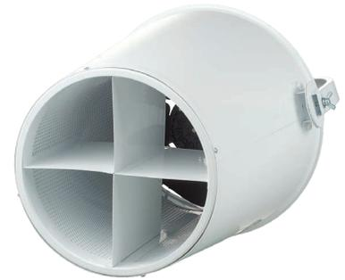
The destratificator is mounted with an arched fixing bracket with position fixation pitch each 15° and a thread-connected mounting and a safety ropes, each 3 m long.
