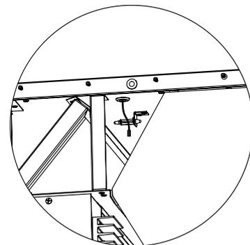
Duct humidity sensor connection
