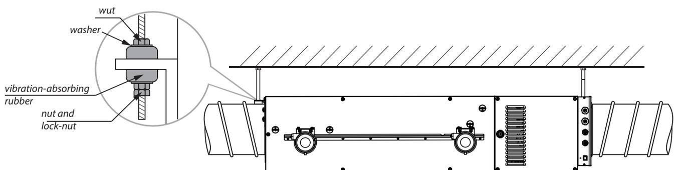
To attain the best performance of the unit and to minimise turbulence-induced air pressure losses while mounting connect a straight air duct section on both sides of the unit.
