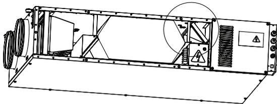
Duct humidity sensor installation place
