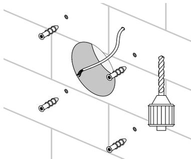
Fix the fan with the screws.
