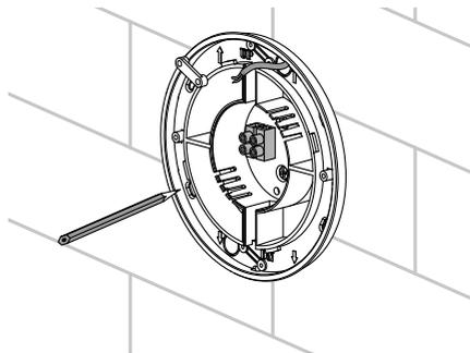
Lead the power cable to the ventilation hole, drill the mounting holes and install the dowels.
