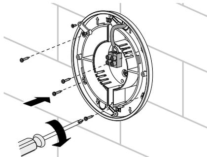
Connect the fan to the electric mains according to the connections diagram. Install the front panel by turning it clockwise. Thread the fixing screw.
