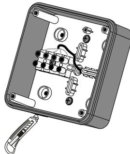
Connect the power cord wires to the terminal block and assemble the fan in reverse order. Supply power to the fan.
