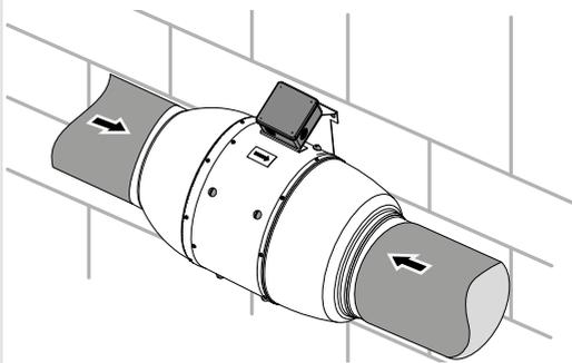
Cut off power supply and make sure electricity has been turned off. Remove the cover of the fan.
