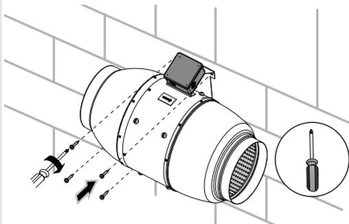
For any mounting position connect an air duct on both sides of the fan.
