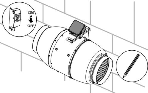
Lead the power cable to the ventilation hole, drill the mounting holes and install the dowels.
