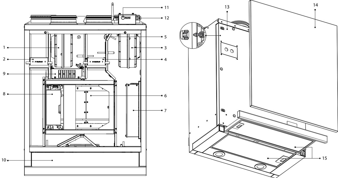
1 — supply fan; 2 — supply filter; 3 — exhaust fan; 4 — exhaust filter; 5 — humidity sensor (optional); 6 — rotary heat exchanger; 7 — control unit; 8 — rotary heat exchanger drive; 9 — electric heater (models equipped with a heater); 10 — cooker hood; 11 — Setup Mode button; 12 — airtight lead-ins; 13 — service panel, 14 — decorative panel (accessory, not included in the delivery set); 15 — cooker hood filters.
