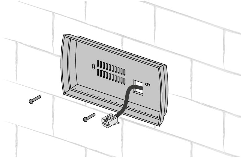
2. Connect the telephone cable to the front side of the control panel. Attach the front side of the control panel to its back side using the supplied countersunk head screws as shown below. Press the control panel front side to click to complete installation.
