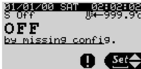
The button will light up. Pressing it displays the alarm code.
