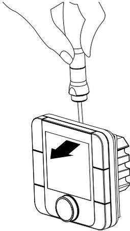
2. Disconnect the 4-pin connector from the front side of the control panel.
