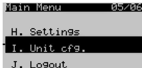
2. In the **Unit cfg.** section, select the **I005 thTune** parameter and change its value from **Y** to **N**.
