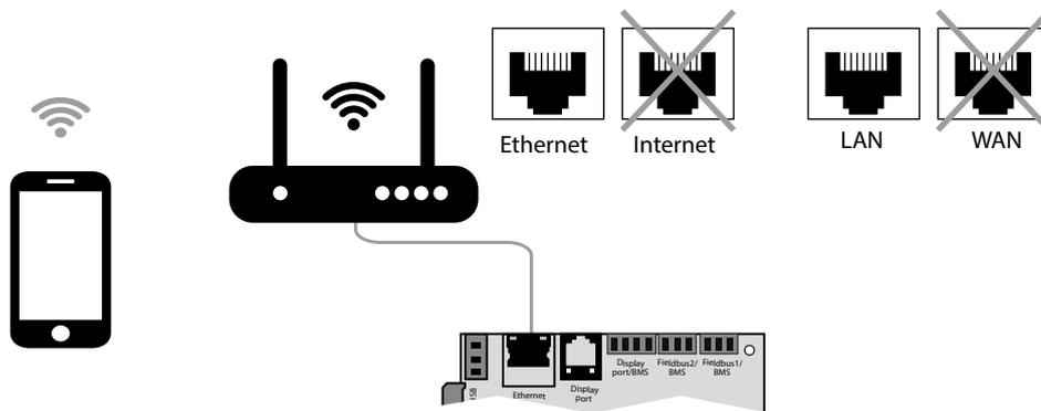
The ventilation unit is controllable via a mobile device or tablet. Connect the router through the Ethernet (LAN) connector using the twisted pair (4 x 2 x 0.51) not below Cat5 with 8P8C connectors. Go to router menu and find IP address of the ventilation unit. Enter IP address in the URL bar in a mobile device.
