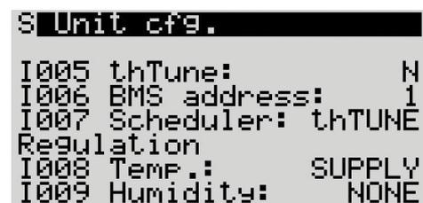
If the control is via **BMS**, the parameter **I005 Enable thTune management** must be set to 0.
