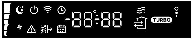
The digital segment of the display shows information such as time, temperature or all the data one by one. The scale on the left shows the fan speed.
