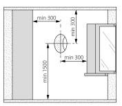
Locate the product as far as possible from heat sources (heating devices, electric stoves, etc.) and devices that use air for combustion (fireplaces, gas stoves, etc.).
