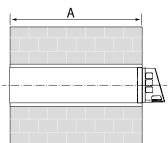
Do not block the air intake grilles or the condensate drain outlet. If necessary, use the supplied mounting wedges (item 3) and sealing foam to ensure that the air duct is fixed in an airtight and immovable manner in the opening.
