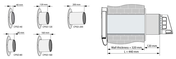
For the most optimal matching of the product length and wall thickness, when access to the outer side of the wall is not possible, take advantage of the trimming option for the outer housing and extension unit of the Breezy Eco 160(-E) L055/L07/L1 models. For wall mounting, use the mounting holes on the compensator pad.
