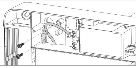
connect the cable to fixed wiring.
