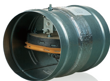
Normally open fire-resisting duct damper with thermal fuse and return spring
