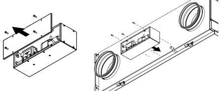
The drainage pump is connected to the power supply and to the sewage system through the product's cable glands according to the user manual for the drainage pump.
