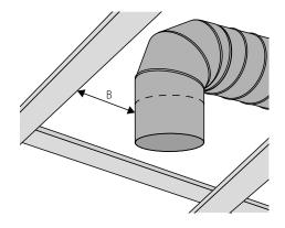
ATTENTION! To prevent vibration, a section of flexible duct must be attached in between the diffuser and rigid duct.
