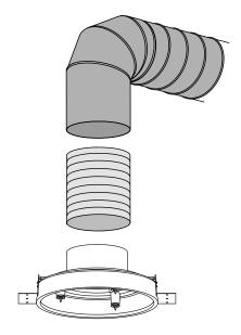
**To attach the mounting brackets to drywall, use screws at least 3.9 mm in diameter. Before starting the installation**, secure the mounting brackets in pre-made holes on the diffuser's casing. Adjust the position of the mounting brackets based on the ceiling thickness (A).
