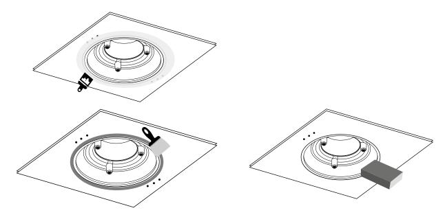
Dust the surfaces and slits. Apply the primer ("Knauf Tiefengrund" or similar). When dry, putty (use "Knauf Fugenfüller" or similar) the slit between the diffuser and drywall. When the spackling paste is dry, grind on the surface.
