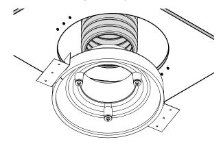
Install the air duct onto the diffuser's flange.
