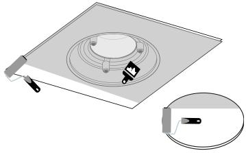
Apply the primer (the one recommended by the paint's manufacturer). Paint the diffuser and the drywall.
