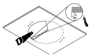
Align the template with the ceiling and mark up the places to install the diffuser and make holes for mounting. Make a hole in the drywall. Remove the chamfer at a 45° angle up to 1/3 drywall thickness.
