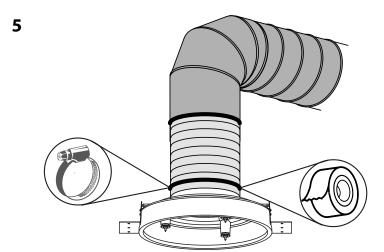
Secure the connection with the worm drive clamp or duct tape.
