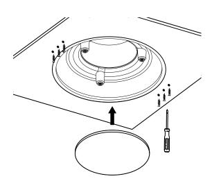
Secure the diffuser with screws. Install the front panel fixed with magnet holders.
