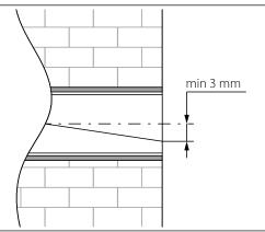
2. Mark the fastening holes for the outer ventilation hood and drill 4 holes, 50 mm deep to suit the expansion anchors (6x40). Use the back wall of the ventilation hood to facilitate the marking.
