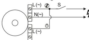
Wiring diagram of the P and P1 fan equipped with a timer/timer and a humidity sensor.
