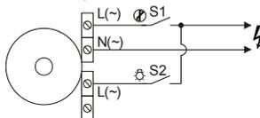
Wiring diagram of the Xstar fan with the simultaneous switching on of the fan and the integrated lamp.
