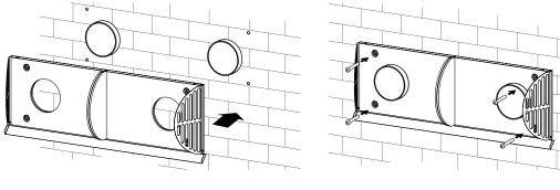
Install the front part of the hood and fix it with screws.
