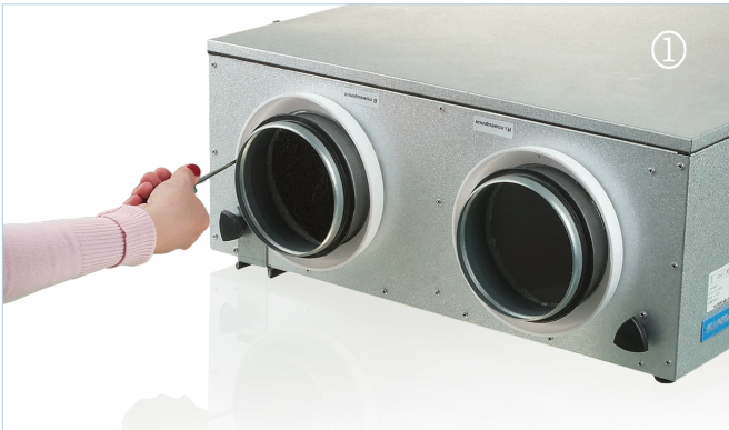
Cover the air handling unit spigots with the flanges from NM Isovent mounting kit and fix those with self-drilling screws with drill.
