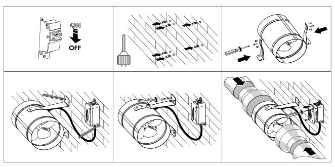
2. Note: the mounting bracket fixing point on the fan casing must be selected so that the screws do not interfere with the free rotation of the impeller.
