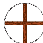
Use of wooden spreader bars during installation
