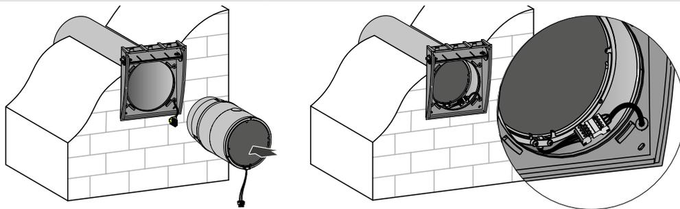
**6. Mount the front panel of the indoor unit and fix the outer ventilation hood.**
