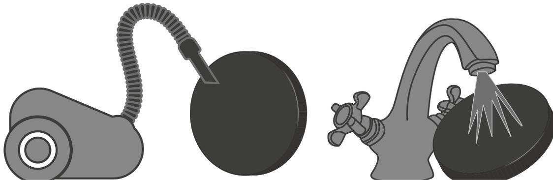
Even regular technical maintenance may not completely prevent dust accumulation on the regenerator and the fan.
