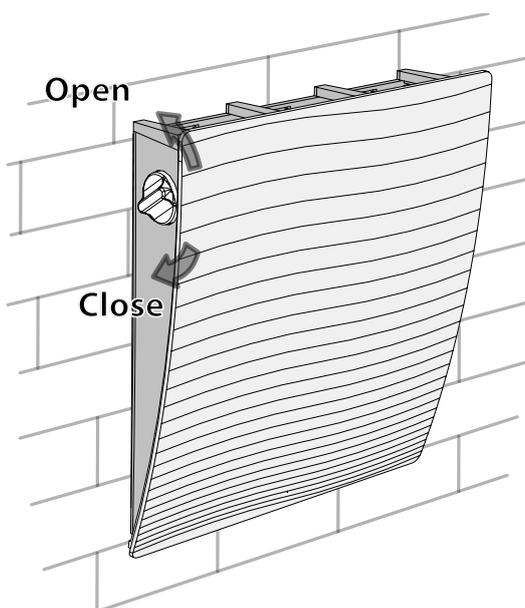
The indoor unit is equipped with a rotary air damper. To open or close the air duct turn one of the levers on the side walls of the indoor unit against stop, as shown below. The vertical lever position corresponds to the OPEN position and the horizontal position corresponds to the CLOSED position.
