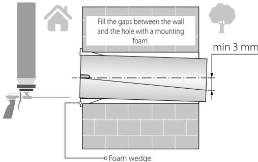
Install the air duct with the minimum slope of 3 mm downwards to the outer wall side using the polystyrene wedges. Fill the gap between the air duct and the opening with mounting foam.
