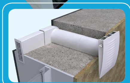
Flush mounting using an NP corner mounting kit
