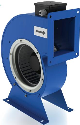
Scroll-type single-inlet centrifugal fans powered by external rotor. Air flow up to **2000 m<sup>3</sup>/h**.
