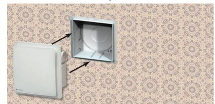
The fan casing is mounted during construction works. Electric wiring for connection of the VNV-1A(E) 80 ventilation unit is led out through a special hole in the casing. The front panel is covered with the protective cardboard plate supplied with the unit to avoid damages or contamination during finishing works in the room. After finishing the works the protective cardboard plate is removed and the VNV-1A(E) 80 ventilation unit is installed into the casing that is connected to the wiring.
