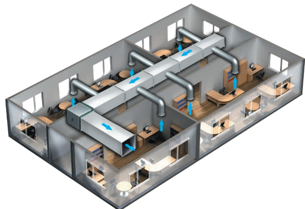
VS fan office ventilation example
