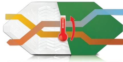
The VUT 2000/3000 PBE/PBW EC units are equipped with a cross-flow plate heat exchanger made of aluminium.
