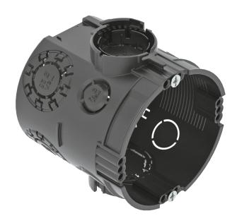
Round mounting box. Recessed box for use in masonry with an installation depth of at least 66 mm. - 4×3 screw caps. - 2 pre-installed screws for devices. - Connector with a bayonet lock that connects on both sides. - 6 combined inlets for pipes  $\emptyset$  20 and 25 mm. - 4  $\emptyset$  20 mm inlets. - 2  $\emptyset$  14 mm inlets. - 1 inlet  $\emptyset$  20 mm at the base. Tested according to DIN EN 60670-1, DIN EN 60670-22 and DIN 49073-1
