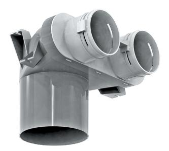
For supply and exhaust systems in residential premises. For under-ceiling mounting with 125 mm duct downwards. Connecting the ventilation grille to  $\varnothing$  90 mm ducts
