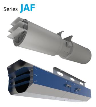
Axial jet fans for ventilation of covered parking. Temperatures of the transported medium: in continuous operation up to +55 °C in smoke extraction mode: 300-400 °C - 2 hrs. Functionality. Power. Efficiency.
