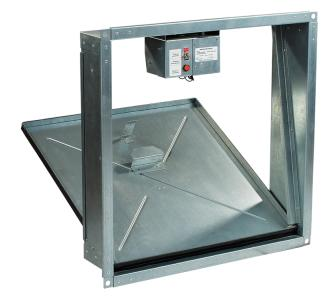
Normally closed single louvre fire safety dampers, fire resistance rating of 180 minutes at smoke temperature of 600  $^{\circ}\text{C}$
