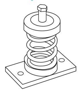
The spring-loaded antivibration mounts are used for attenuation of noise and vibration generated by ventilation equipment
