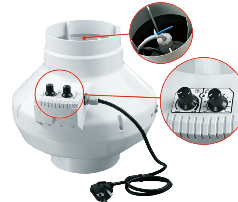
VK ... U built-in speed control module with thermostat and integrated temperature probe, power cable with EURO-plug
