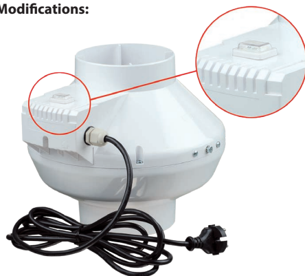
VK ... Duo R1 double-speed motor, built-in speed switch (high speed/OFF/low speed), power cable with EURO-plug
