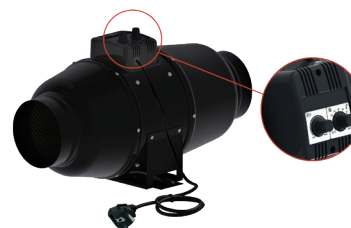
TT Silent-M ... U built-in speed control module with thermostat and integrated temperature sensor, power cable with EURO-plug
