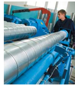
Spiral wound ducts workshop
