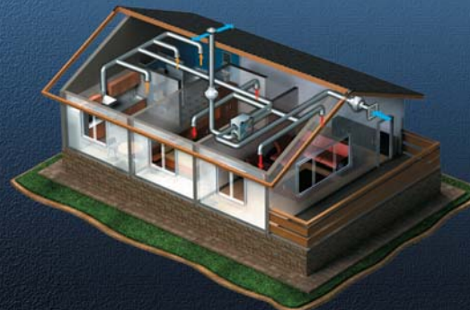
Installation Vents PR 150 in room ducting
