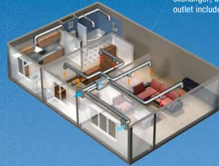
Installation Vents VUE 150 P mini in room ducting
