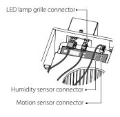
4. Install the decorative grille on the fan casing using the holders on the casing.
