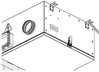
**3.** Fix the fan on the mounting brackets using the appropriate fasteners.
