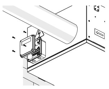
2. Drill the holes according to the markings.
