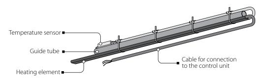
Adjust the heater length L in consideration of the air duct length and the vent hood dimensions.
