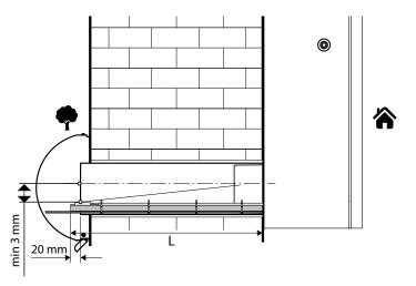
Mark the necessary length of the heater L on the guide tube, cut off the extra cable ties with wire cutters, move the cable away to the side and saw off the redundant part of the tube.
