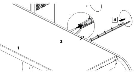
To access the control unit, open the air handling unit and remove the shielding plate by undoing the attachment screws.
