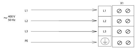
The electric parameters of the fan are shown on the label on the fan casing. For the fan modifications without a terminal box, connect the cable directly to the fan motor. Connection sequence: remove the protective hood (item 3, fig. 3, 4) after removing the screws (item 9, fig. 3, 4) which fix it. After finishing wireworks re-install the protective hood.
