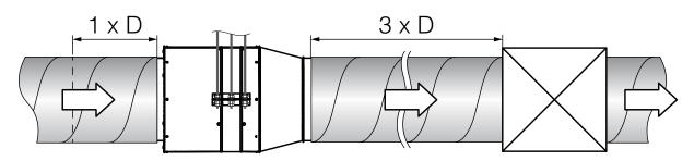
To attain the best performance of the fan and to minimise turbulence-induced air pressure losses connect the straight air duct section to the spigots on both sides of the unit while mounting.
